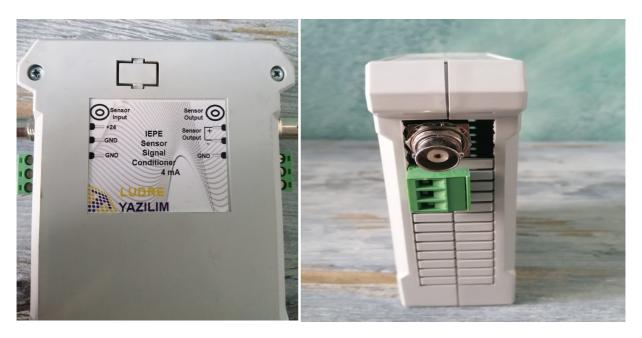
We connect the input section with BNC cable between IEPE Microphone and IEPE Sensor Signal Conditioner. then we make the 24V dc connection for the system to work. From the output part of the conditioner, we connect it to a software/screen where we can see the harmonic sound waves with a BNC cable. and the IEPE Microphone is ready to use.
