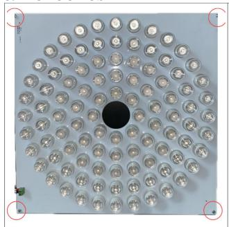
Mounting to the machines is possible with the bolt and nut assembly in the areas indicated in the adjacent image. The points to be taken into consideration during this installation are as follows: The electronic parts should not be contacted while assembling the product. In addition, if the product is not installed properly, vibrations that may occur will cause errors during measurement and control.
