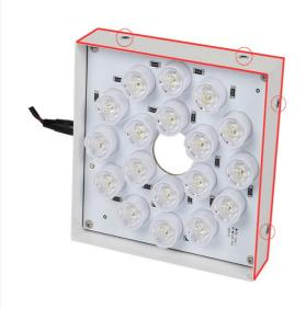
There are guides in the areas indicated in the figure. You can mount it in these areas with fasteners such as M4 bolts and nuts. There are 12 connection points that you can mount, which are not shown in the image.
